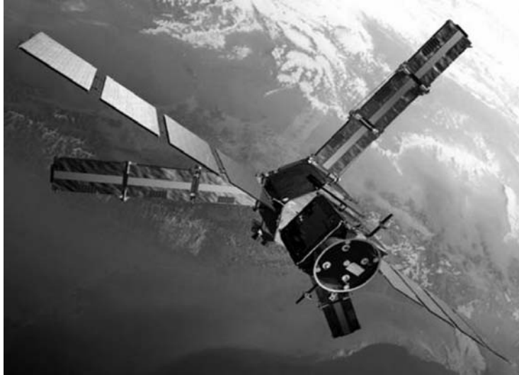
Figure 1. SMOS artist view with the three arms deployed forming a Y-shaped structure. The total number of receiving elements in the interferometric radiometer is 69 (image courtesy of ESA Medialab).
